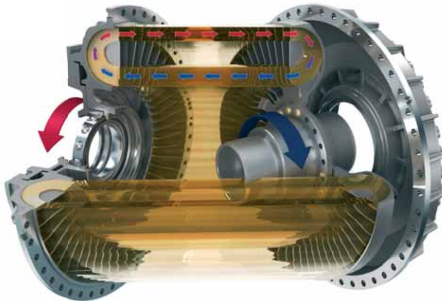
Fig. 14: 3-D sectioned model of a hydrodynamic constant-fill coupling with fluid distribution during start-up
